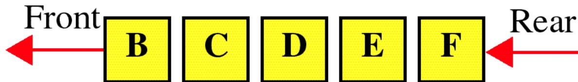
b. After removing first element
